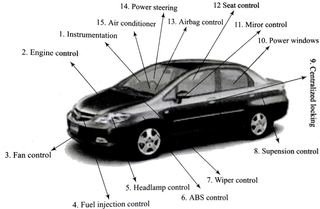
Embedded System in the Automotive Domain
